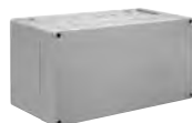
Electric junction box with mains adapter 100 – 240 V. 50 – 60 Hz, 9 V, for 1 – 12 solenoid valves Item No. 01 583 00 99
